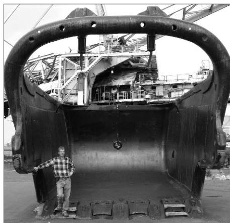
Author John Hiemstra stands inside a dragline bucket, used in mining oil sands.
